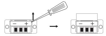
5. Turn the terminal screws counter-clockwise to loosen
